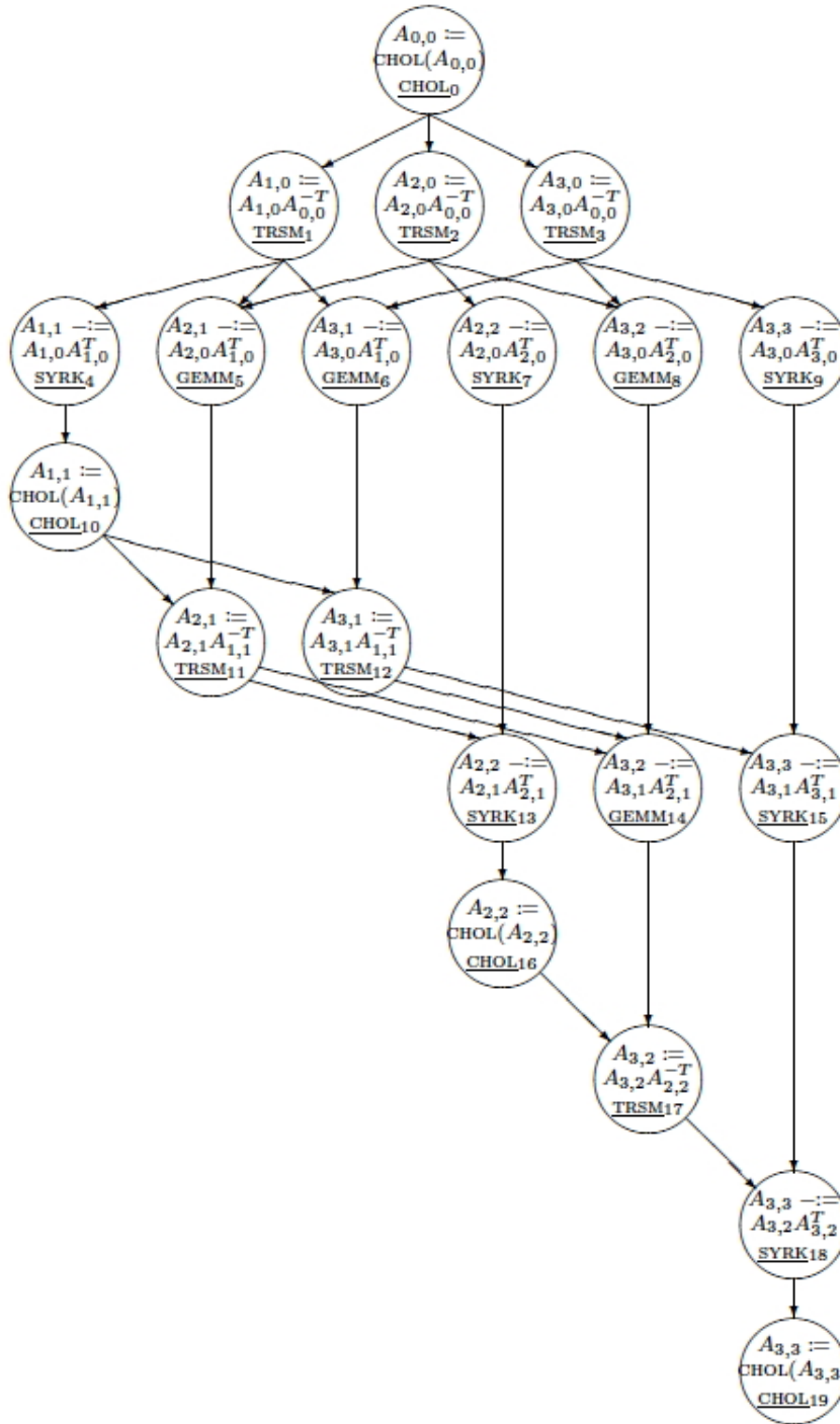
Figure 6.24: Graph of task dependencies in a 4 \times 4 Cholesky factorization
