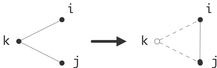
Figure 5.3: Eliminating a vertex introduces a new edge in the quotient graph
