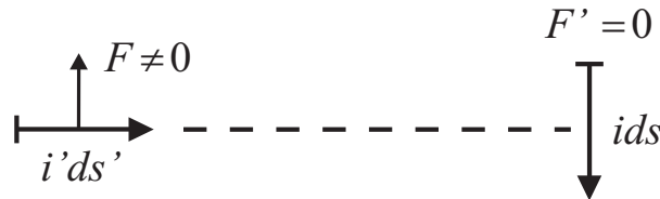
Figure 20.8: Two orthogonal elements. Grassmann's force F exerted by ids on i'ds' is different from zero, while Grassmann's force F' exerted by i'ds' on ids is zero.
