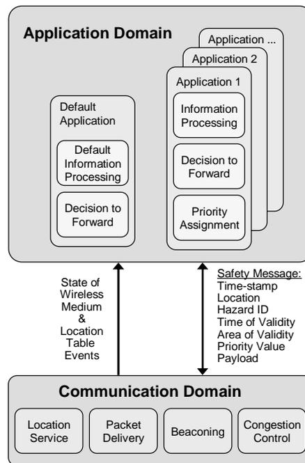
Figure 7.4: High level view of the proposed model for IVC nodes.
