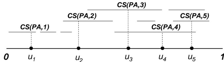
Figure 5.1: Network load based on carrier sensing: the maximum load is experienced in  $R = [0, 1]$  where the number of intersecting carrier sensing ranges is maximal. In the example, we have  $BL(PA, 5) = 3$ .
