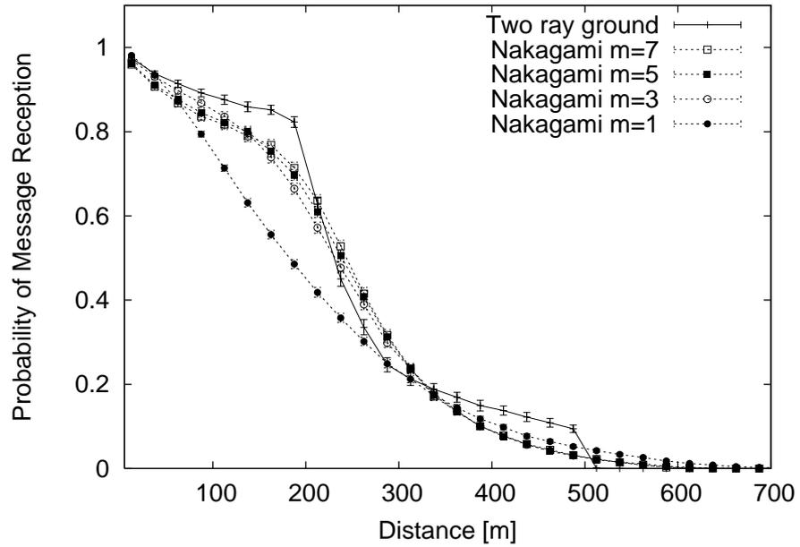
Figure 3.8: Probability of successful beacon reception with respect to the distance in a 3-lane per direction highway scenario with 66 vehicles/km. Comparison of the results obtained by using different propagation models with a data rate of 6 Mbps, an intended communication range of 500 m and a packet generation rate of 10 pkts/s.
