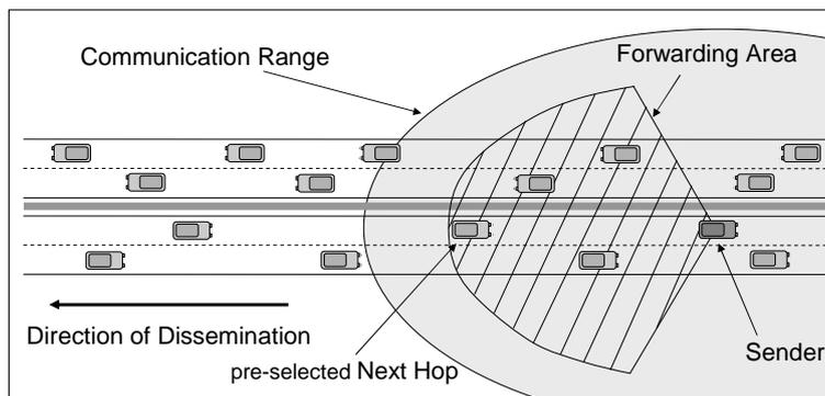
Figure 5.6: Illustration of the sender perspective when utilizing the EMDV protocol.
