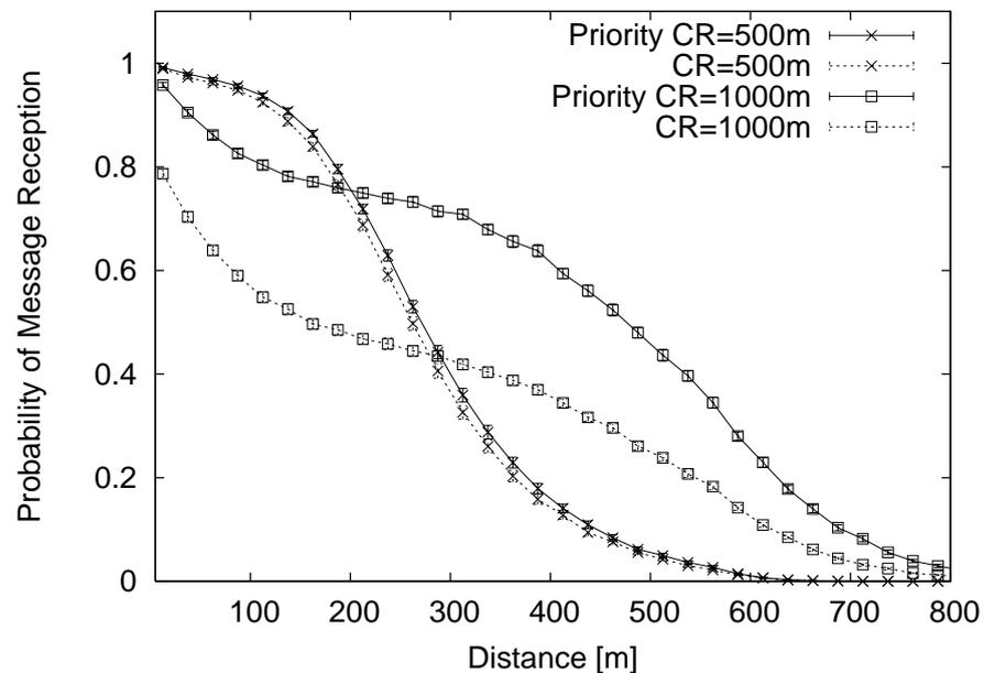
Figure 3.11: Probability of successful beacon reception with respect to the distance in a 3-lane per direction highway scenario with 66 vehicles/km. Comparison of the results obtained by a priority and non-priority node with different communication ranges, a data rate of 3 Mbps, a contention window of 31, and a packet generation rate of 10 pkts/s.
