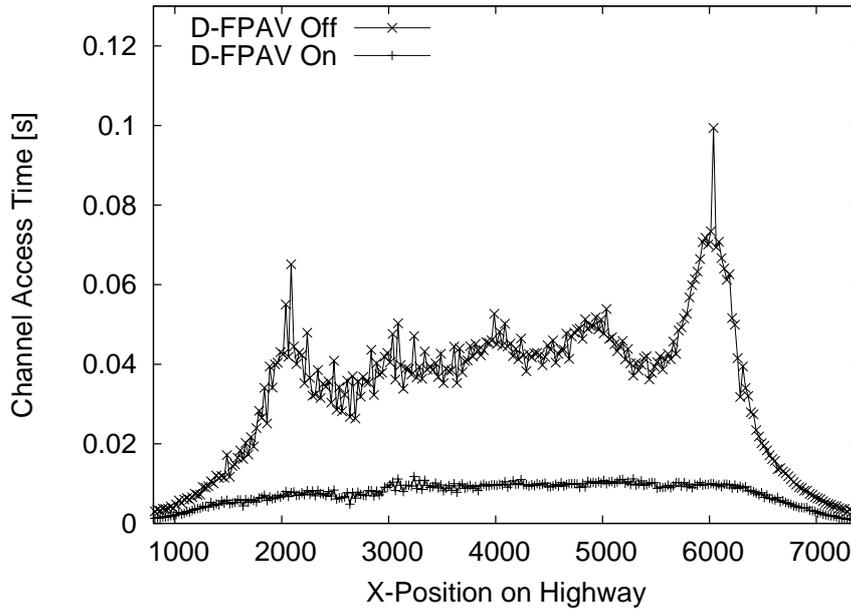
(a) Average channel access time experienced by each node with respect to its position on the highway.
