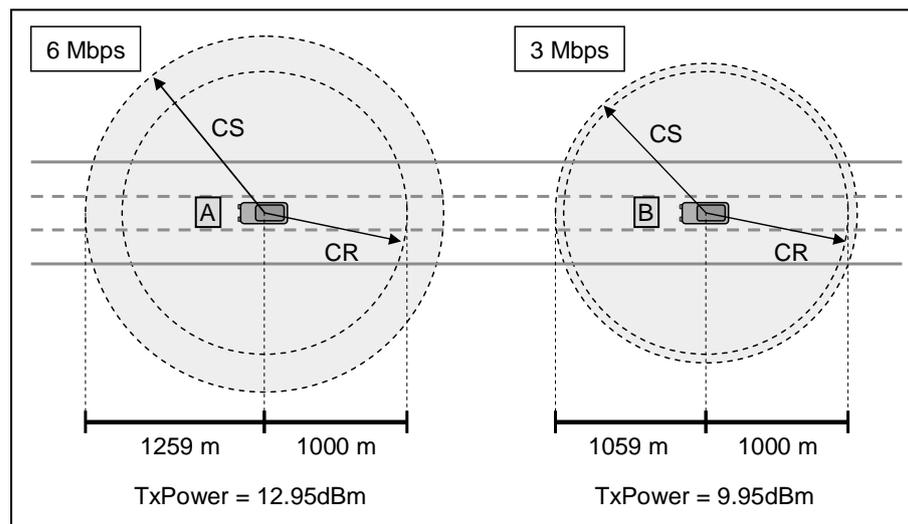
Figure 3.2: Communication and carrier sense ranges obtained for a signal transmitted power of 12.95 dBm with a data rate of 6 Mbps, and 9.95 dBm with a data rate of 3 Mbps.
