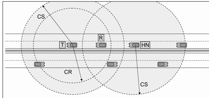
Figure 3.7: The hidden node (or terminal) problem: In a CSMA/CA scenario assuming a deterministic propagation model, node R is inside the Communication Range of T and node HN is placed outside of the Carrier Sense range (CS) of T, i.e., HN can not sense ongoing transmissions from T. In that case, the hidden node problem occurs when T’s message is interfered by an HN’s transmission at R’s position.
