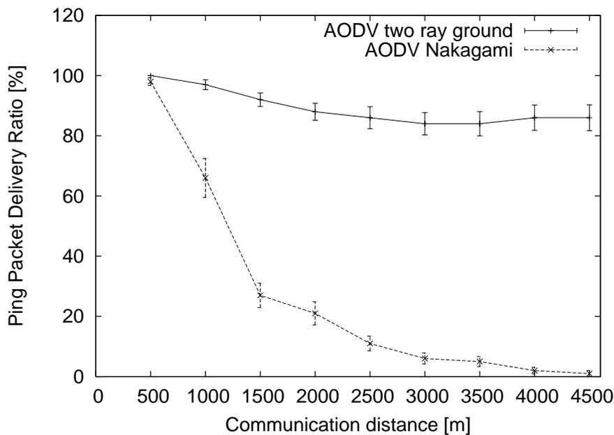
Figure 4.2: Ping message delivery ratio in a multi-hop highway scenario with a connected network and utilizing AODV, a communication range of 500 m, and the propagation models of two ray ground and Nakagami. Values presented with a 95% confidence interval.
