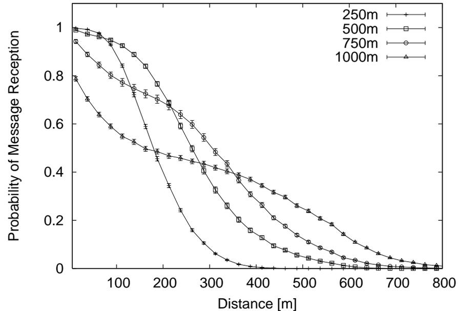
Figure 3.10: Probability of successful beacon reception with respect to the distance in a 3-lane per direction highway scenario with 66 vehicles/km. Comparison of the results obtained by using different communication ranges with a data rate of 3 Mbps, a contention window value of 31 and a packet generation rate of 10 pckts/s.
