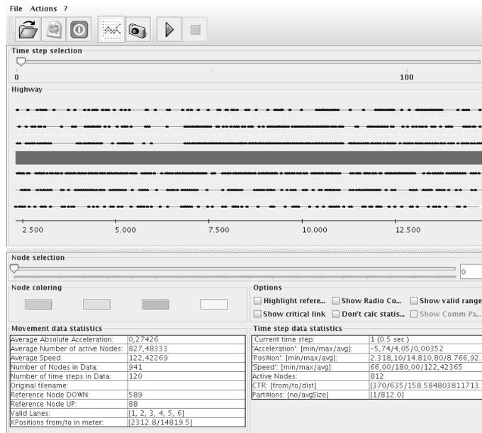
Figure 3.4: Screen-shot of the HWGui tool [FTMK<sup>+</sup>06] with a scenario composed of 3 lanes per direction and 6 nodes per kilometer in each lane.
