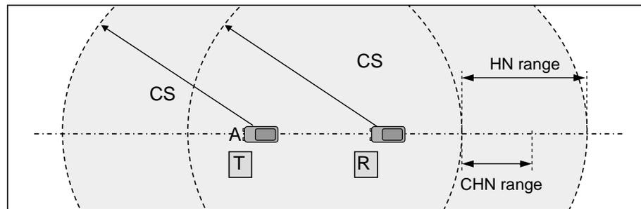
Figure B.3: Illustration of the HN (Hidden Nodes) range and the CHN (Colliding HN) range.
