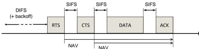
Figure 2.4: Unicast channel reservation and acknowledgment exchange scheme.
