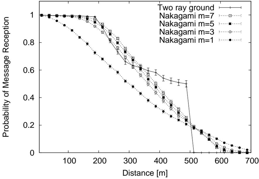
Figure 3.6: Probability of successful beacon reception with respect to the distance in a 3-lane per direction highway scenario with 36 vehicles/km. Comparison of the results obtained by using different propagation models with a data rate of 6 Mbps, an intended communication range of 500 m and a packet generation rate of 10 pkts/s.
