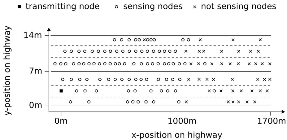
Figure 4.1: The node represented with a black square, transmits one message to the channel with an intended CR range of 1000 m, what corresponds to a CS of 1059 m. Using the non-deterministic Nakagami radio propagation model, with an  $m$  parameter set to 3, white circles represent nodes that sense the message on the medium and 'x's represent those which do not.
