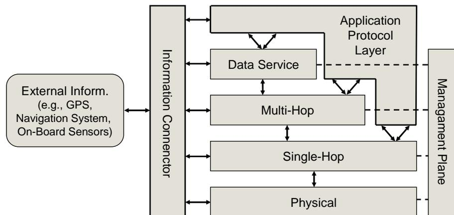
Figure 7.3: Sketch of the proposed protocol architecture for inter-vehicle communication systems.
