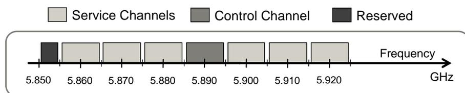
Figure 2.1: Spectrum allocation for intelligent transportation systems in the USA.
