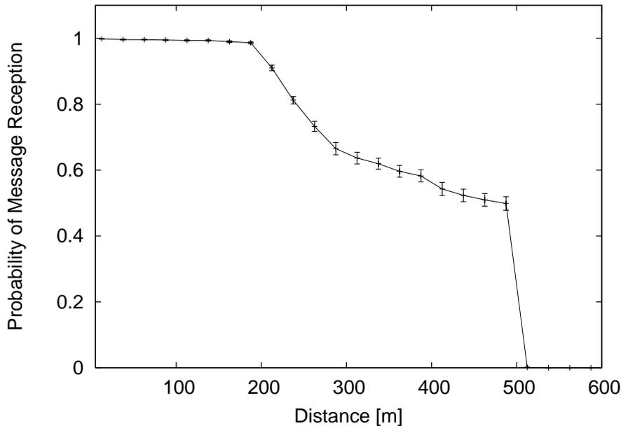
Figure B.2: Probability of successful beacon reception with respect to the distance in a 3-lane per direction highway scenario with 36 vehicles/km, data rate of 6 Mbps, intended communication range of 500 m, packet generation rate of 10 pckts/s and the two ray ground model.
