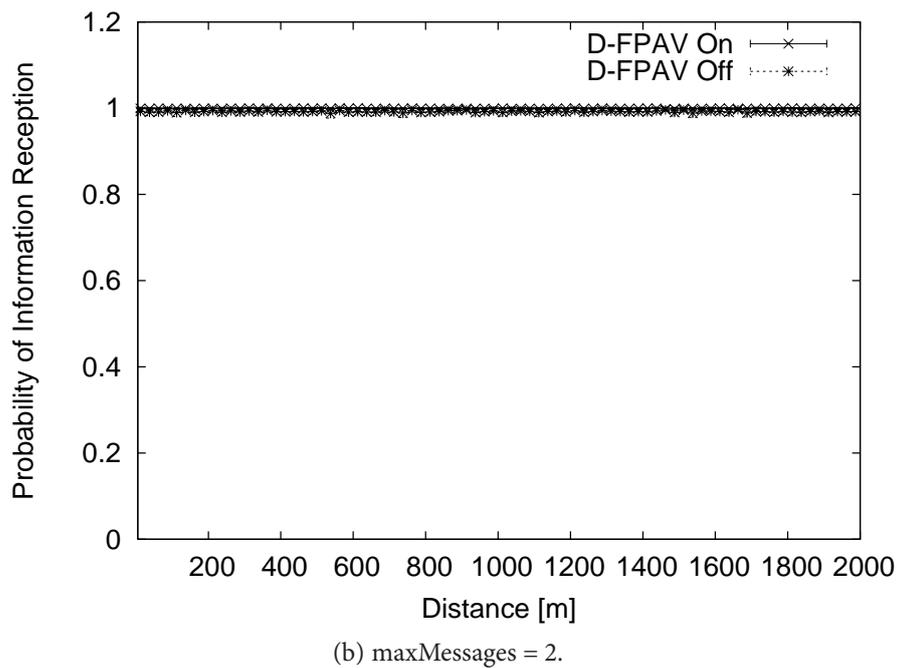
Figure 6.5: Probability of information delivery inside the dissemination area with respect to the distance from the message originator (with multi-hop retransmissions) with D-FPAV On/Off and MBL = 2.5 Mbps.
