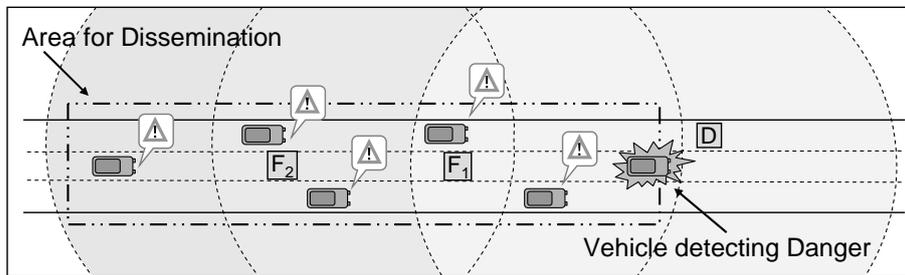
Figure 2.7: Exemplary road situation where vehicle D detects a hazard and issues an event-driven message. Vehicles  $F_1$  and  $F_2$  forward the message to cover the area of dissemination where the information is relevant. The shaded circles represent the direct communication ranges of the nodes originating and forwarding the event-driven message, D,  $F_1$  and  $F_2$ .
