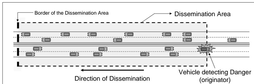
Figure 5.5: Relevant area for dissemination of emergency information after an accident detection in a highway. Vehicles in the opposite direction are included in the dissemination area since they can support the dissemination process.
