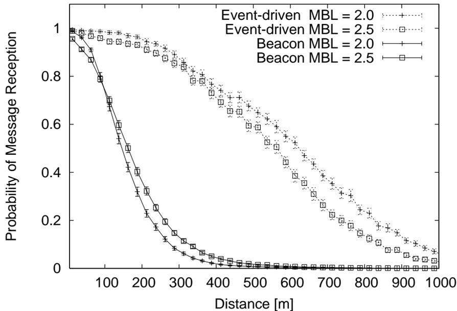
Figure 6.8: Probability of successful reception with respect to the distance of beacons and one hop event-driven messages (without retransmission) with D-FPAV On for MBL=2.0 Mbps and MBL=2.5 Mbps.
