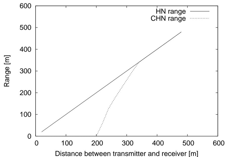
Figure B.4: HN and CHN ranges with respect to the distance between the transmitter and the receiver.
