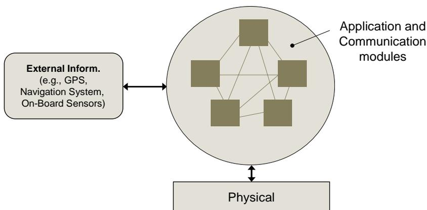
Figure 7.2: Un-layered approach for an IVC system.
