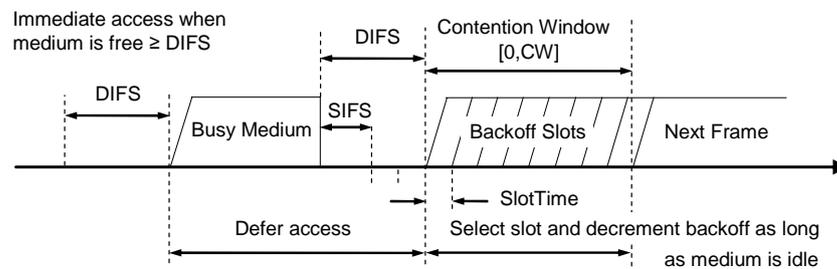
Figure 2.3: Distributed coordination function for channel access.
