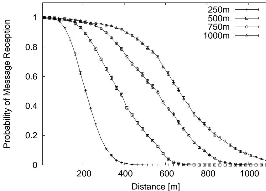
Figure 3.12: Probability of successful beacon reception with respect to the distance in a 3-lane per direction highway scenario with 36 vehicles/km. Comparison of the results obtained by using different communication ranges with a data rate of 3 Mbps, a contention window value of 31, and a packet generation rate of 10 pckts/s.
