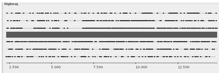
Figure 6.1: Screen-shot of the HWGui tool [FTMK<sup>+</sup>06] corresponding to a utilized highway scenario, with 3 lanes per direction and 11 nodes per kilometer in each lane.
