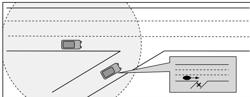
Figure 2.6: Exemplary road situation where the existence of periodic messages can assist the driver in low visibility conditions. The vehicle entering the highway is aware of the near vehicle when it receives a beacon. The shaded circle represents the direct communication range of the vehicle driving on the highway.
