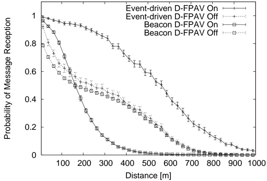
Figure 6.3: Probability of successful reception of beacons and one hop event-driven messages (without retransmission) with respect to the distance to the transmitter, with D-FPAV On/Off and MBL = 2.5 Mbps.
