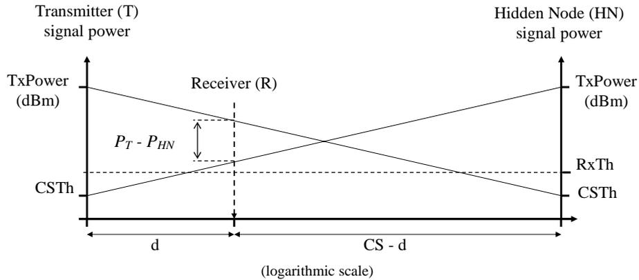
Figure B.1: Illustration of the ‘robust range against hidden nodes’ with a deterministic propagation model.
