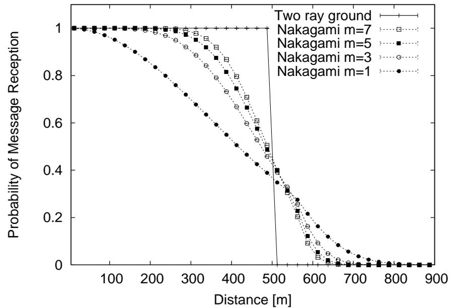
Figure 3.5: Probability of successful packet reception without interferences from other nodes with respect to the distance with a transmission power corresponding to a CR of 500m with a data rate of 6 Mbps and different radio propagation models.
