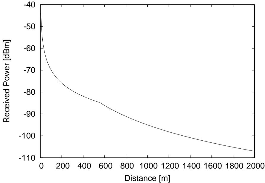
Figure 3.1: Received signal power with respect to the distance to the transmitter computed by the ns-2.28 implementation of the two ray ground propagation model.
