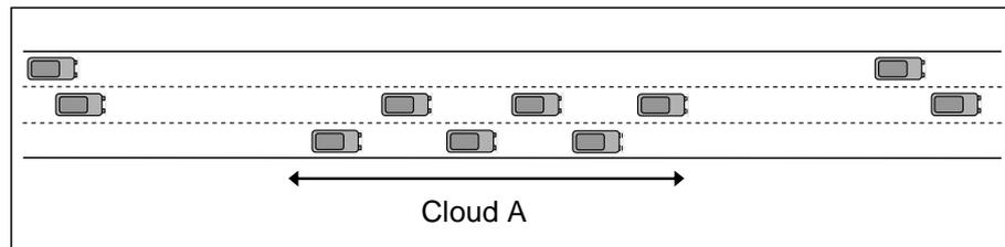
Figure 4.4: If nodes forming Cloud A would try to optimize capacity they would adjust their transmit power to reach only the closest car [GK00]. In this case, they would not have direct awareness of the next vehicle in the same lane even though it is very close.
