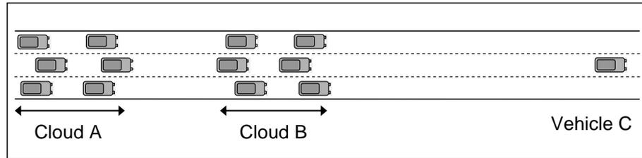
Figure 4.3: If nodes from Cloud B would try to be connected with far away Vehicle C, they can create a high level of interference disturbing information exchange among vehicles inside Cloud A.
