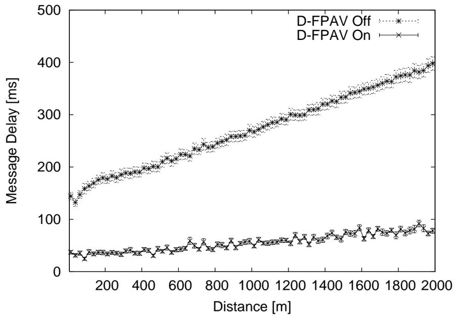
Figure 6.7: Reception delay of the emergency information inside the dissemination area with respect to the distance from the message originator (with multi-hop retransmissions) with D-FPAV On/Off and MBL = 2.5 Mbps.
