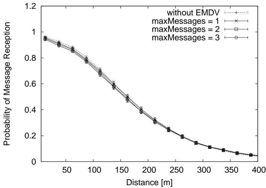
Figure 6.6: Probability of successful reception of beacons with respect to the distance, with D-FPAV On, MBL = 2.5 Mbps and while disseminating emergency information for three values of *maxMessages*, 1, 2 and 3.
