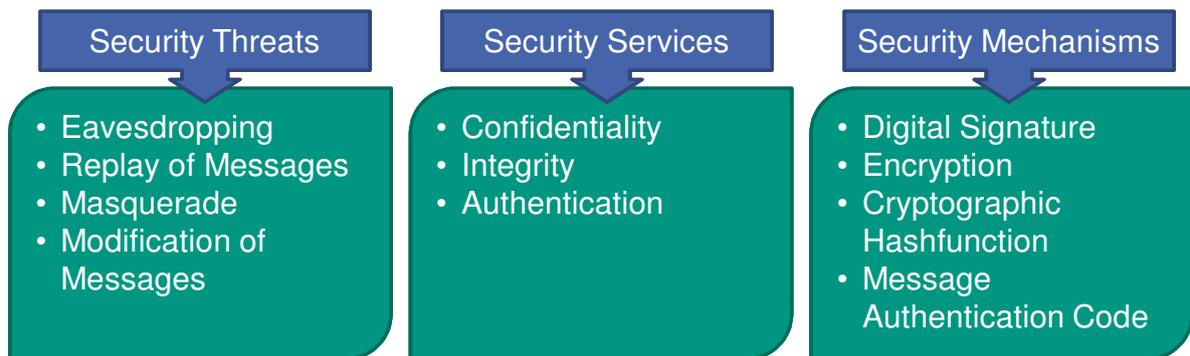
**Figure 3.3:** Signaling protocols can use a specific set of security mechanisms in order to realize security services and protect from security threats
