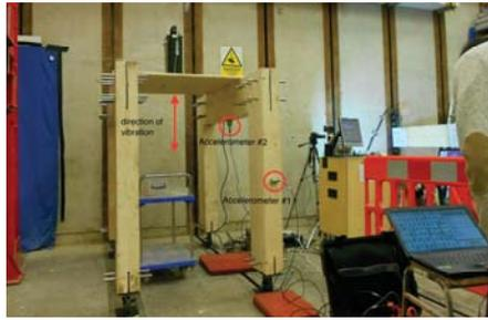
Figure 8. Portal frame under vibration test.
