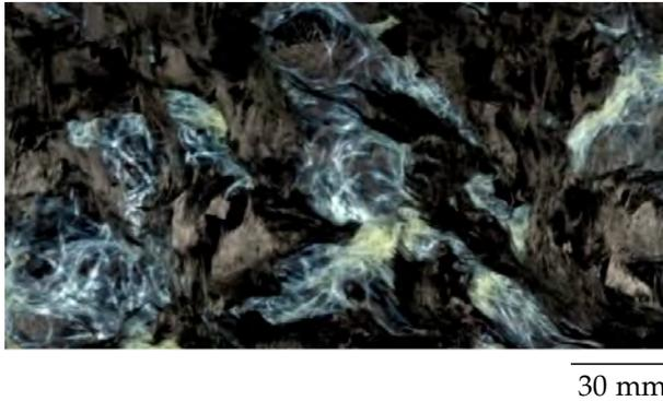
**Figure 2.22:** Hybrid glass/carbon fibre reinforced SMC sheet in interlayer configuration based on stacking of chopped glass and carbon fibres reinforced semi-finished sheets prior to moulding and manufactured within the framework of the IRTG (GRK 2078).
