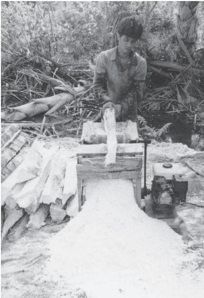
Figure 3.2. Mechanized grinding (*mengolah sagu*) in an outdoor “sago factory.” (Photograph by Wini P. Utari)
