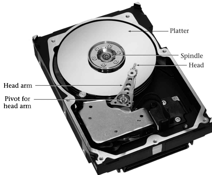
Figure 8.1 In this photo of an opened disk drive, a stack of four platters is visible at the top, with a head arm extending into the platter area. The part you can see is the topmost layer of the head arm, holding the head for the top surface of the top platter. Similar layers are stacked below it; for example, the next layer down has heads for the bottom of the top platter and the top of the second platter. Photo copyright by and reprinted by courtesy of Seagate Technology LLC.
