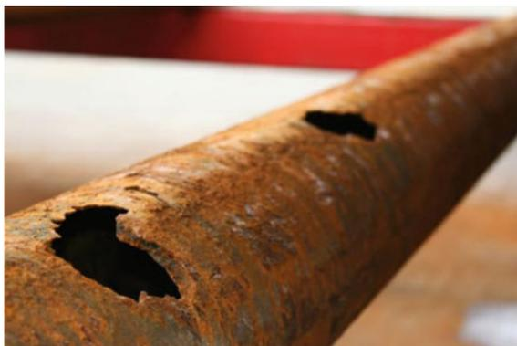
bridge plug which has been installed in tail pipe of production tubing. The bridge plug is going to be pressure tested and therefore, a fluid is injected through the production tubing. A corroded production tubing with holes exposes the production casing to high pressure and consequently, the casing may burst due to the imposed pressure. Therefore, good knowledge of production tubing condition is necessary prior to starting the P&A operation.
