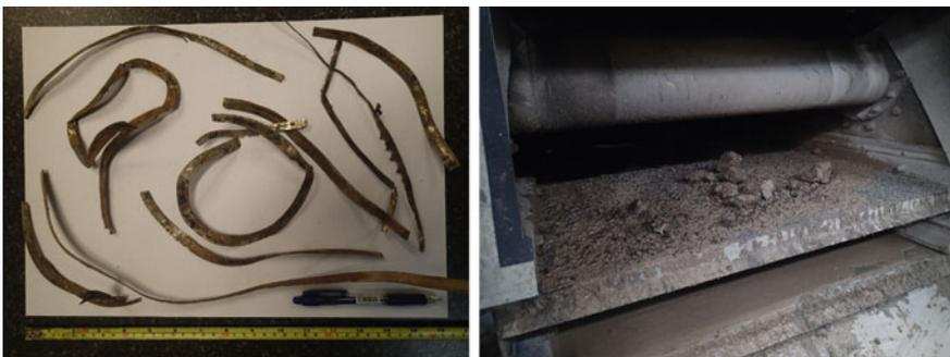
Fig. 7.1 Swarf from a milling operation in the North Sea (Courtesy of equinor)
