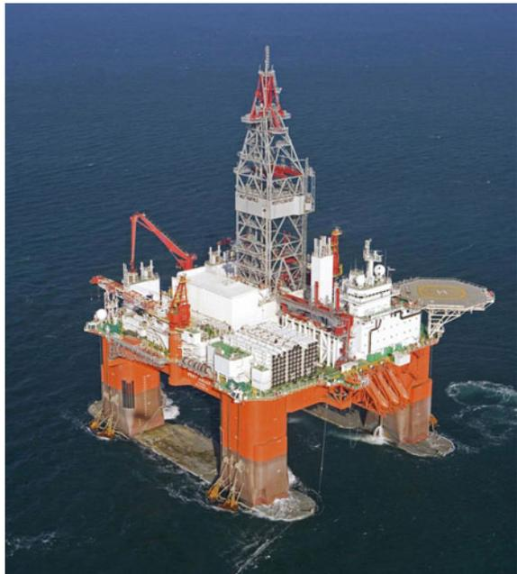
rest on the seafloor, the unit is either *anchored* onto the position or kept on location with dynamic positioning systems. The construction and operational cost of semisubmersible rigs are higher than for submersible rigs.
