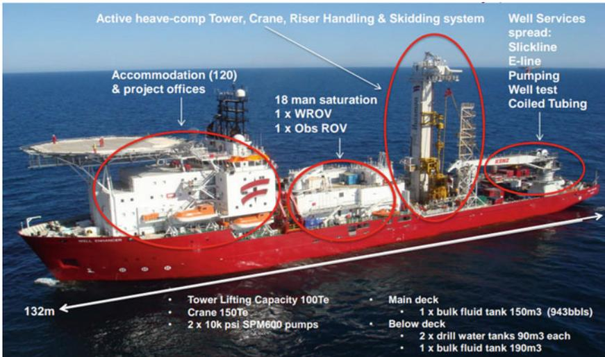
Fig. 5.8 Light well intervention vessel. (Courtesy of Helix Energy Solutions Group)
