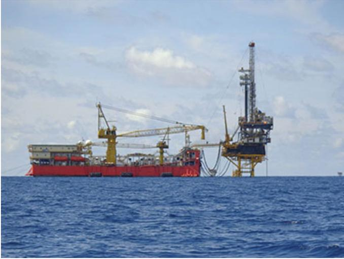
**Fig. 5.7** A tender rig in operation while the anchored vessel is in service. (Courtesy of Seadrill)
