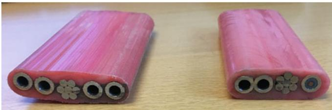
Fig. 2.29 Control lines with and without electrical line
