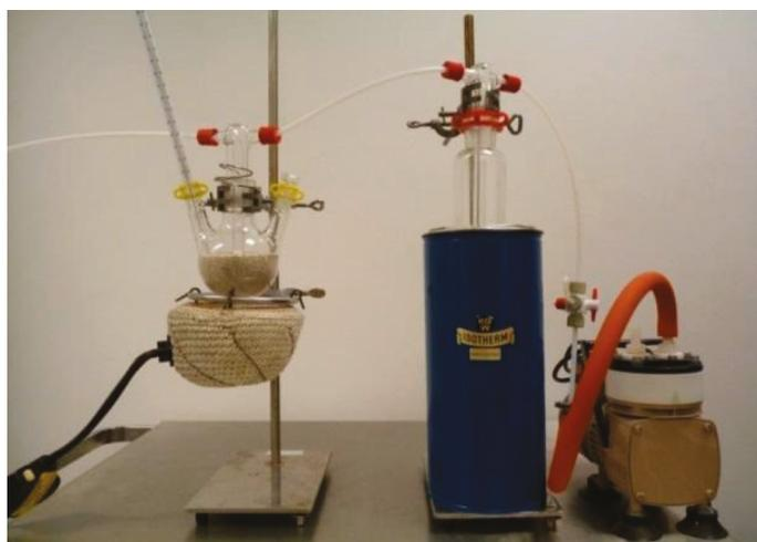
**Figure 4.** Condensation unit for the recovery of  $[^{18}\text{O}]$ -water from azeotropic mixtures.
