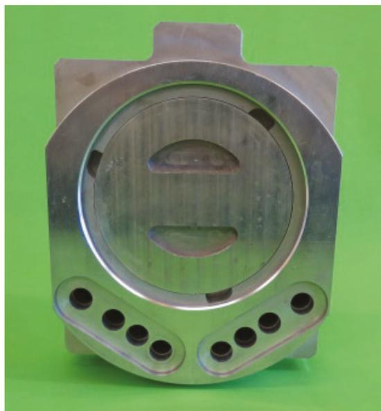
Figure 8. A closed tandem target holder with the bayonet-mount plug in position.
