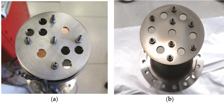
**Figure 2.** Masks assembled on heated substrate-holder for Mo sputtering (a) and on nonheated substrate-holder for Y sputtering (b).
