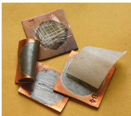
Figure 4. Tests for adhesion of coatings.
