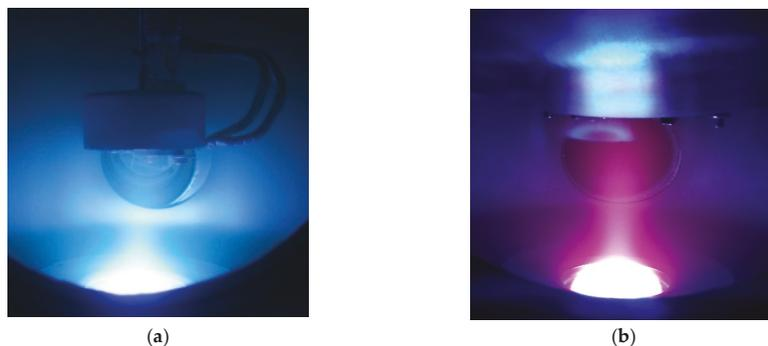
Figure 4. Plasma of Mo (a) and Y (b) during the sputtering process.
