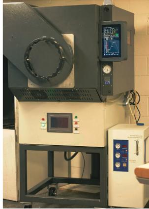
Figure 1. Hydrogen oven and H<sub>2</sub> generator.
