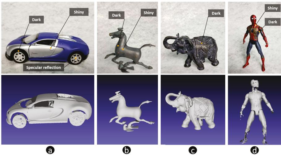
**Figure 13.** Experimental results of the proposed hybrid measurement approach. (a) plastic surface with shiny, dark and specular reflection regions; (b) metal surface, which results in shiny and dark regions from different perspectives of observation; (c) stone material with very low reflection; (d) plastic surface with multiple reflectance and large variation of normal directions.
