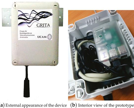
**Figure 5.** Views of the physical prototype built. (a) Final design of the acoustic device. In the picture, the Raspberry Pi and the other components are inside a protected box. At the bottom part of the box, the microphone can be observed; (b) Interior view of the waterproof case. The components inside of it are the Raspberry Pi together with the POE splitter, the microphone at the bottom of the picture and all the cables for the connection.
