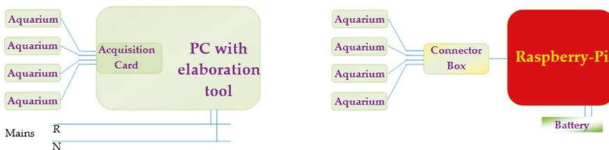
Figure 9. Classical and Raspberry-based architecture.
