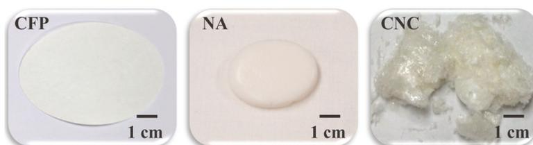
**Figure 1.** Images of the cellulosic (CFP) and nanocellulosic (NA and CNC) transducers.
