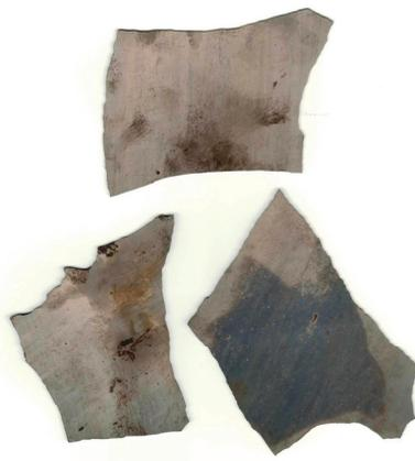
Figure 7. Electrolytic manganese flakes.
