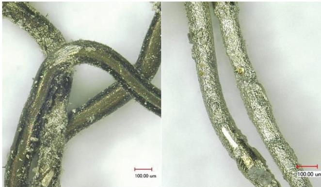
**Figure 7.** Silver cementation on nickel threads.
