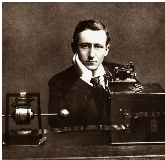
FIG. 20.3 'Transfer between Boxes'. Guglielmo Marconi (1874–1937) pictured between the spark-gap transmitter on the right and the coherer receiver on the left. Together he and Karl Ferdinand Braun were awarded the Nobel prize in physics in 1909 (source: Google-hosted LIFE Photo Archive)
