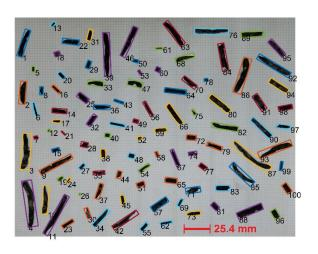
Figure 15 - Burning sticks were captured and quenched in pans of water. Dimensions of each captured firebrand (N = 1155) were measured using a calibrated image.
