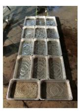
Figure 8 - Water pan arrangement for firebrand collection.
