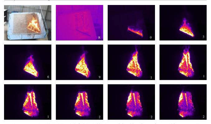
Figure 5 - Test AVE08 ( $\alpha$ =30°;  $\gamma$ =20°;  $\delta$ =45°): visible picture of the table, reference frame and frames every 30 seconds, from instant 0s to 270s.
