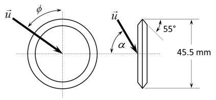
Figure 3 - Diagram of the front and side views of disks with some arbitrary wind vector.
