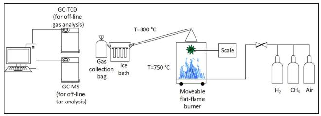
Figure 1 - Flat-flame burner setup used to measure pyrolysis products resulting from heating southern wildland fuels at a high heating rate.
