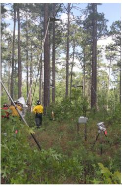
Figure 2 - In-situ infrared tripod system, FPBs and video sensors.
