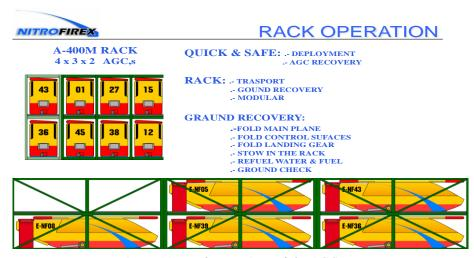
Figure 11 - Rack operations of the AGCs.
