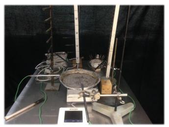
Figure 4 - P. halepensis' litter burning device.
