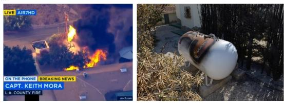
Figure 2 - Left: Calabassas fire (California, 2016). A propane jet fire can be observed at the centre of the image. Flames from ornamental fuels are close to the tank. LPG infrastructure was inside a kindergarten facility. Right: Domestic LPG tank in Benitatxell (Spain, 2016) damaged by the jet fire. The tank was surrounded by an ornamental hedgerow that ignited by spotting.
