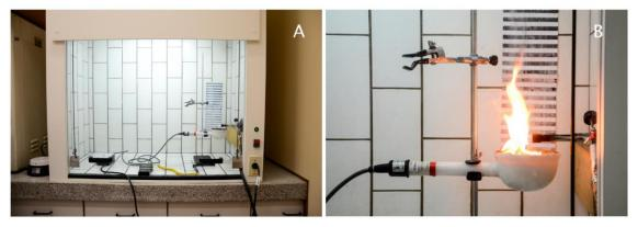
Figure 1 - Epirradiator in the fume hood (A) and epirradiador test (B)
