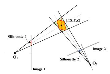
Figure 5 - Simplified 2D sketch illustrating the visual hull method for 3D particle shape reconstruction (only 2 cameras considered here; O<sub>i</sub>: camera perspective centers, X, Y and Z: 3D coord. of the particle centroid).
