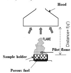
Figure 1 - A schematic representation of the experimental setup.
