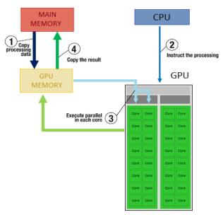
Figure 2 - General workflow of a GPU program
