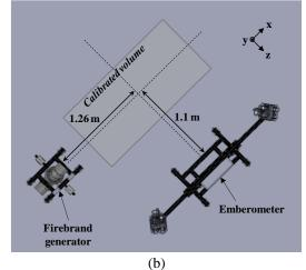
Figure 6 - Experimental layout for tests at the National Fire Research Laboratory (blower and ignition loop of the firebrand generator not shown here): (a) 3D view; (b) Top view with characteristic dimensions
