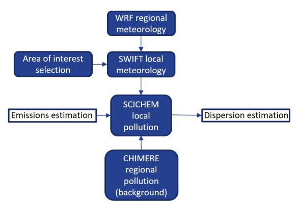
Figure 3 - Dispersion module workflow
