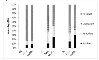
Figure 7 - The comparision between tube furnace and muffle furnace
