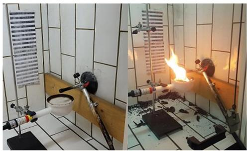
Figure 1 - Epirradiador in the test chamber and in operation.gure
