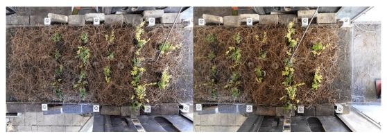
Figure 6 - Vertical stereo photographs of wind tunnel fuel bed used to provide 3D image.
