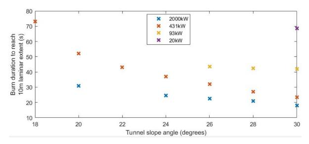
Figure 4 - Simulation time taken for flame attachment to work its way up the escalator trench to point when its laminar boundary layer depth was squeezed out to the trench sides, or 10m for the geometry of the tunnel trench considered.
