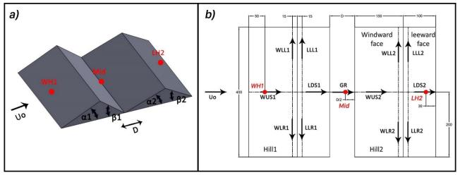
Figure 1 - a) Schematic view of the two triangular hills with the terminology configuration parameters b) Plan view of the used model size with the directions used to evaluate the ROS of the fire. The three ignition points that were used are labelled in red. The dimensions are indicated in cm.
