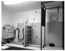
Figure 1 - Radiative Heat Flux Apparatus
