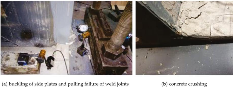
**Figure 5.** Buckling of side plates, pulling failure of weld joints, and concrete crushing of flat steel plate-concrete shear wall (SPSW) specimens with small holes.
