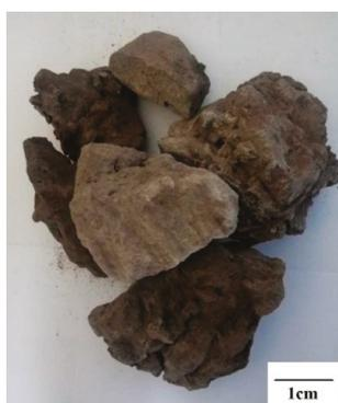
Figure 1. Deposition samples of RHF waste heat recovery system.
