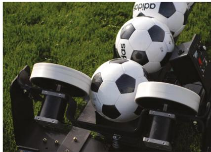
Figure 5. Mechanical inertial rotating launcher.
