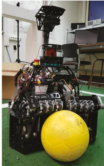
**Figure 30.** RoboCup robot for testing the optimized coil gun.
