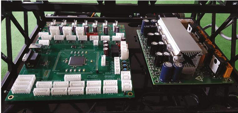
Figure 31. Four-channel reluctance coil gun driver (on the right).
