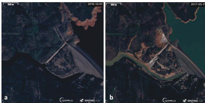
**Figure 3.** Oroville dam, California, USA, (a) before and (b) after the spillway incident occurred in February 2017, in two satellite multispectral images collected on 1 December 2016 and 11 March 2017, respectively (contains Copernicus Sentinel-2 data 2016–2017). The full time-lapse is provided in the Supplementary Materials.
