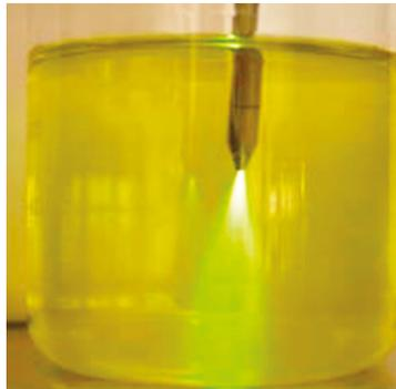
Figure 6. Tyndall effect, 10 ppm fluorescein sodium in water [4].
