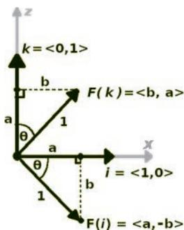
FIGURE 3.17 Calculating rotation around the  $y$ -axis.
