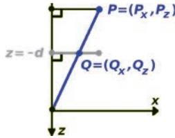
FIGURE 3.25 Calculating  $x$ -components of projected points.
