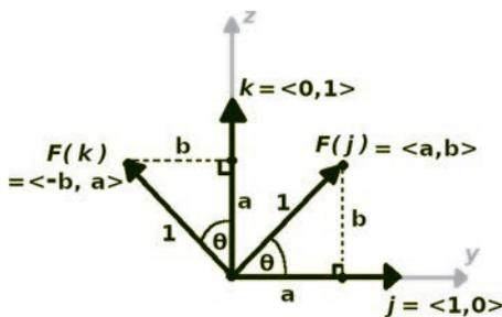
FIGURE 3.16 Calculating rotation around the  $x$ -axis.
