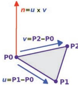
FIGURE 6.10 Calculating the normal vector for a triangle.
