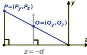
FIGURE 3.24 Calculating  $y$ -components of projected points.
