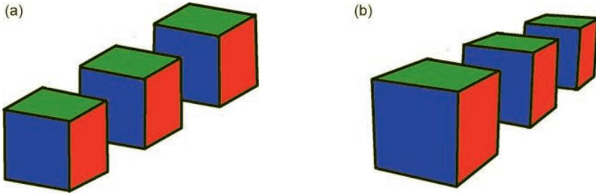
FIGURE 1.11 A series of cubes rendered with orthogonal projection (a) and perspective projection (b).
