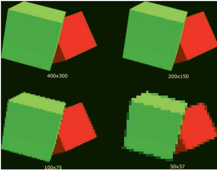
FIGURE 1.5 A single image rendered with different resolutions.
