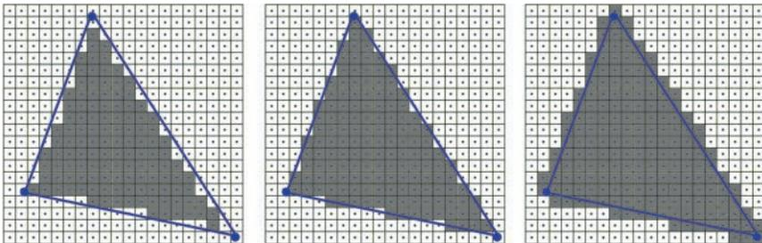
FIGURE 1.12 Different criteria for rasterizing a triangle.
