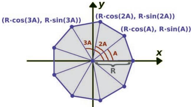
FIGURE 4.11 Calculating the vertices of a regular polygon.
