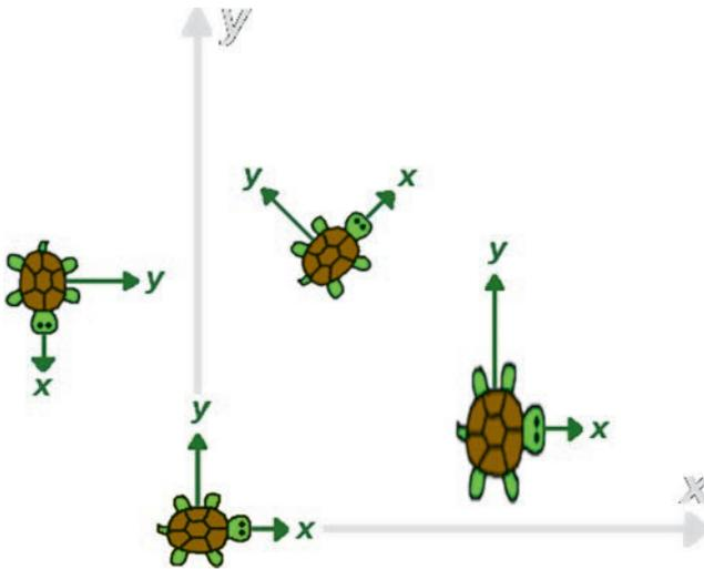
FIGURE 3.27 Transforming local coordinate axes.
