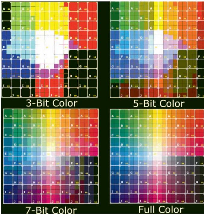
FIGURE 1.6 A single image rendered with different precisions.
