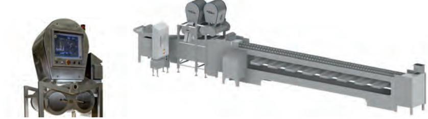
Figure 2.1: Ripening sorter using Sherlock Food Analyzer and eight ejection units.
