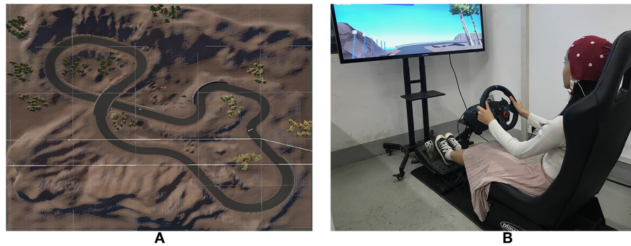
FIGURE 1 | Simulated driving system. (A) driving track, (B) simulated driving platform. The participant has provided written consent for the publication of this image.
