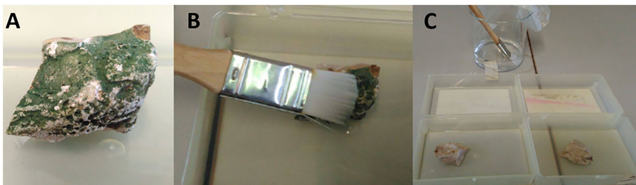
FIGURE 7 | Sample from the Santa Margherita's cave (A), treatment with Preventol RI-80 at 10 v/v %. (B), and application of the CRS (C).
