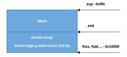
When CAN\_USE\_HEAP is not set, we just use a minimal stack from \_end to \_end + STACK\_SIZE:
