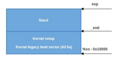
• In the second scenario, ( ss != ds ). First of all put the \_end (address of end of setup code) value in dx and check the loadflags header field with the testb instruction to see whether we can use the heap or not. loadflags is a bitmask header which is defined as:
