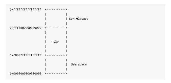
This solution is sign extension. Here we can see that the lower 48 bits of a virtual address can be used for addressing. Bits 63:48 can be either only zeroes or only ones. Note that the virtual address space is split into 2 parts:
