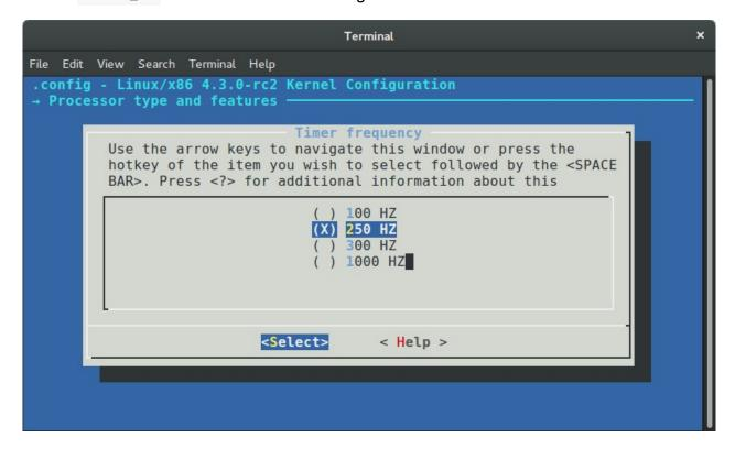
This means that in our case the timer interrupt frequency is 250 Hz or occurs 250 times per second or one timer interrupt each 4ms.
