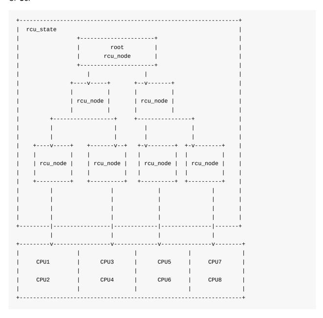
So, in the rcu\_init\_geometry function we just need to calculate the total number of rcu\_node structures. We start to do it with the calculation of the jiffies till to the first and next fqs which is force-quiescent-state (read above about it):
