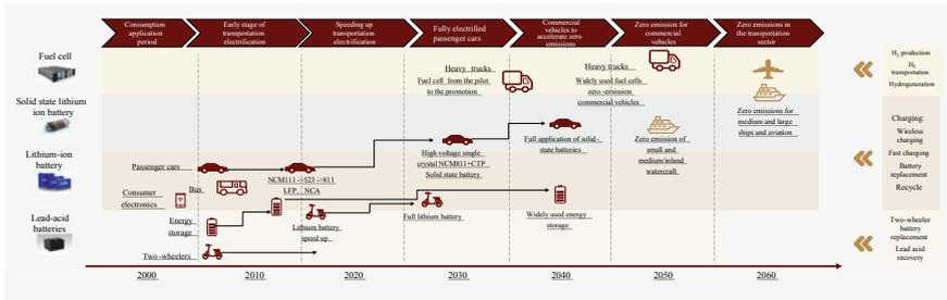
Fig. 8.7 Technologies used in the transportation industry. *Source* GGII, CICC Research
