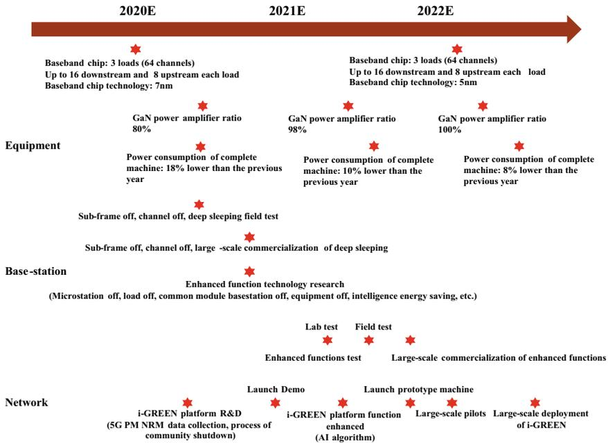
Fig. 11.3 Timeline of energy-saving technologies for 5G base stations. Source CMRI, CICC Research
