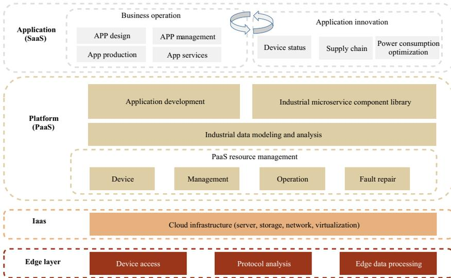
**Fig. 11.1** Architecture of the industrial internet platform. *Source* Industrial internet platform whitepaper released by Alliance of Industrial Internet in 2017, CICC Research. *Note* SaaS refers to software as a service, PaaS refers to platform as a service, IaaS refers to infrastructure as a service
