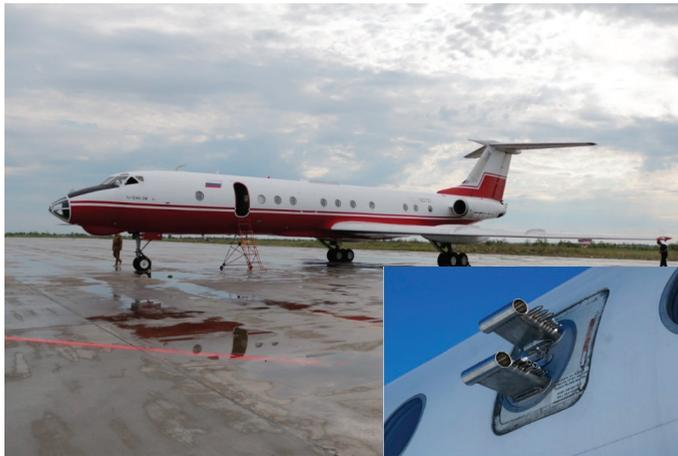
**Figure 2.** Photo of Tupolev-134 aircraft. Insert is the samplers' Inlets.
