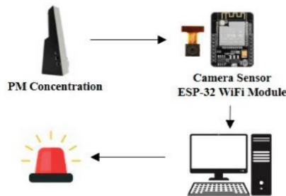
**Figure 5.** Overview of the data communication module system.
