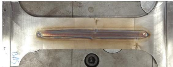
Figure 3. Welded PVR specimen after the experiment.
