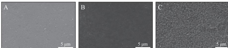
**Figure 2.** Representative SEM micrographs displaying the surface morphology of HA and SiHA thin films where (A) is an as deposited thin film on a CPTi substrate, (B) annealed at 600 °C in flowing argon for 2 h and (C) 700 °C in flowing argon for 2 h. Images taken from HA samples.
