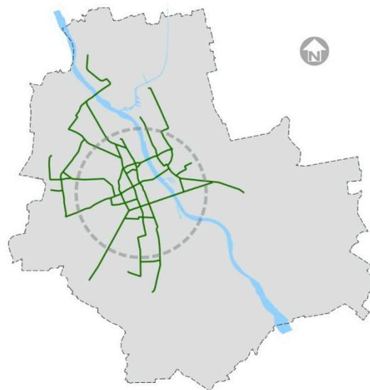
Figure 11. Diagram of the tram system in Warsaw with the central zone of the city. Compiled by P. Wiśniewski, 2021.
