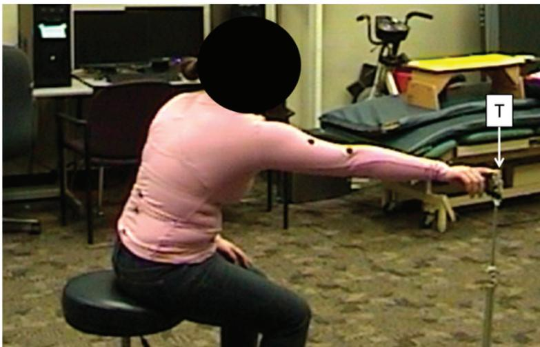
**Figure 1.** An example of a participant reaching towards the target (T) during an extended scaption reach while wearing retroreflective markers.
