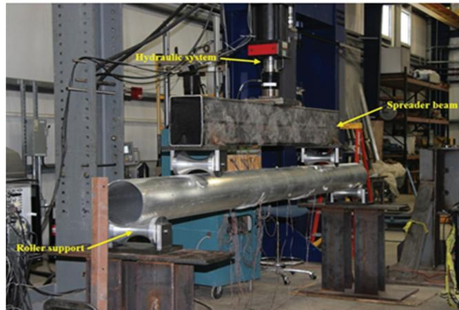
**Figure 3.** Four point bending fatigue test set-up.
