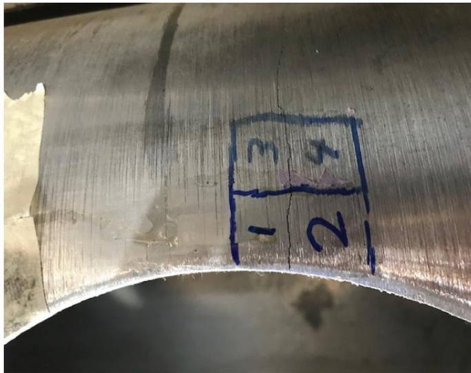
**Figure 10.** Fatigue crack through pole.
