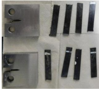
**Figure 3.** Specimens ready to be glued with carbon fiber-reinforced polymer (CFRP) patches (strips).
