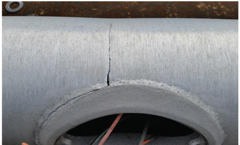
**Figure 1.** Aluminum light pole containing a fatigue crack within the field.
