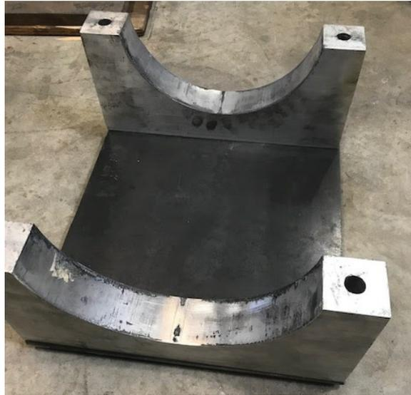
**Figure 5.** Half of the moment clamp used to reinforce the hand-hole after initial failure.
