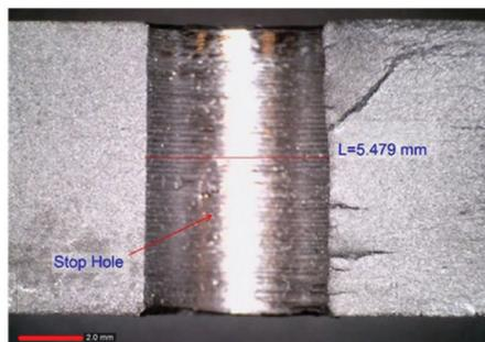
**Figure 9.** Specimen after stop hole technique testing procedure with re-initiated crack after the hole (crack growth direction from left to right).
