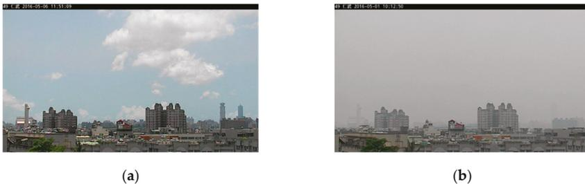
**Figure 3.** A sample image pair. (a)  $I_1$  (low PM<sub>2.5</sub> concentration, 1 µg/m<sup>3</sup>); (b)  $I_2$  (high PM<sub>2.5</sub> concentration, 75 µg/m<sup>3</sup>).
