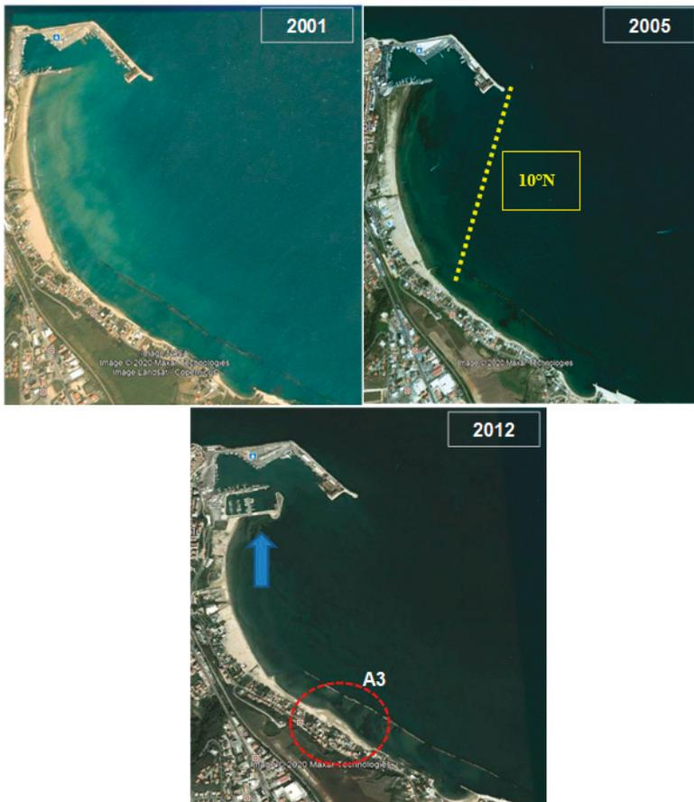
**Figure 8.** View of the area A3. Yellow dotted straight line represents sheltering by  $10^{\circ}$  N waves. (Section 5).
