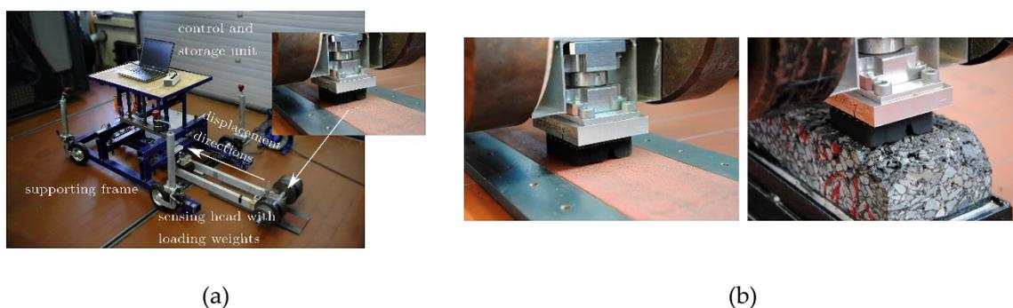
**Figure 21.** (a) LiRep general view (left); (b) detail of two different road surface configurations [70].**Table 11.** Technical specification of the LiRep device.
