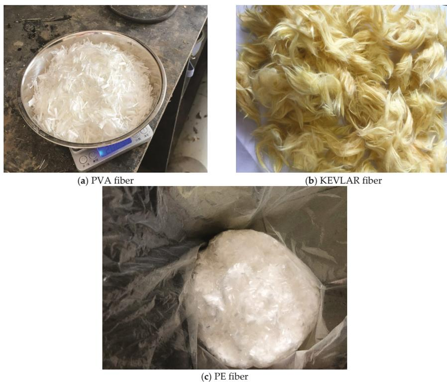
**Figure 1.** Three types of fibers used in the current study. (a) PVA fiber; (b) KEVLAR fiber; (c) PE fiber.
