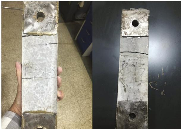
Figure 5. Post-failure specimens of steel grid-PVA fiber reinforced ECC with multiple cracks.
