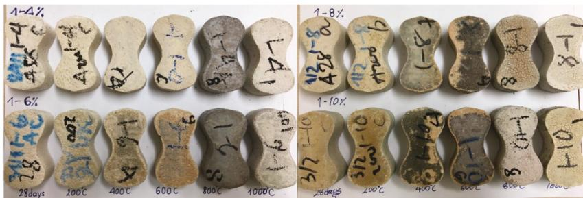
Figure 4. Photographs of AAS mortar samples activated with different concentration of Na<sub>2</sub>O before and after exposure to high temperatures from 200 to 1000 °C.
