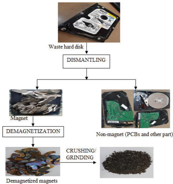
Figure 1. Pre-treatment of magnets prior to leaching of REMs.
