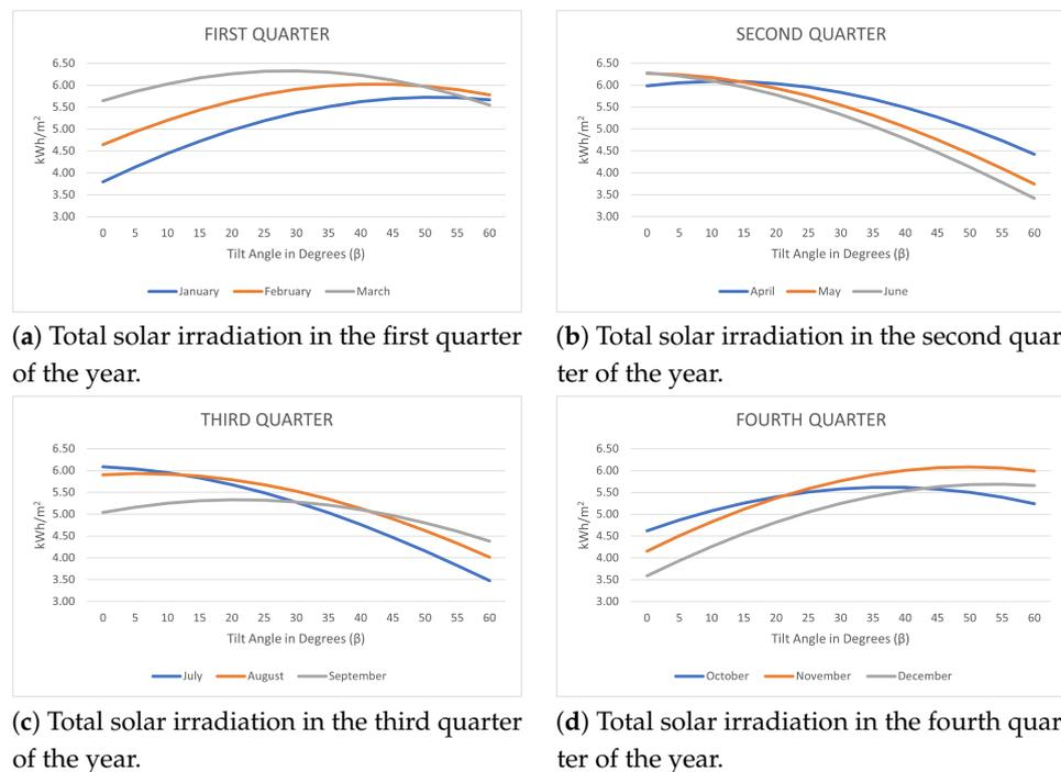
**Figure 4.** Total solar irradiation throughout the year in kWh/m<sup>2</sup>, depending on the tilt angle when azimuth equals 0, broken down into quarters.
