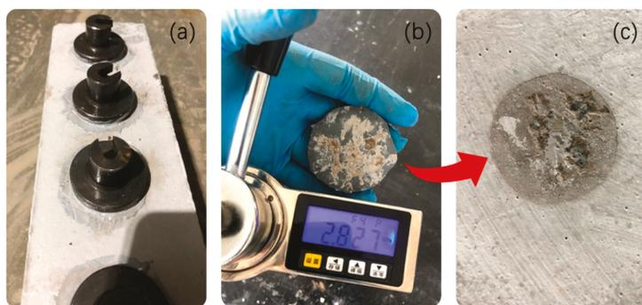
**Figure 4.** Adhesive strength test of GPC: (a) standard steel flanges glued on the surface of GPC layer that was previously coated on concrete substrate; (b) pulling out steel flanges from glued GPC surface with a portable adhesion tester, the LCD screen displays adhesive strength (MPa) of GPC; (c) failure interface between GPC layer and concrete substrate.
