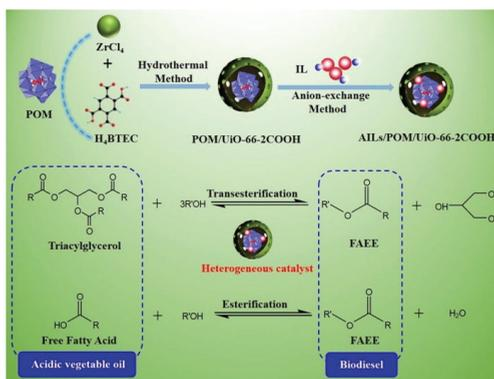
**Figure 9.** Synthesis procedure of the AILs/HPW/UiO-66-2COOH catalyst, and one-pot transesterification-esterification of acidic vegetable oils. Reprinted from [114]. Copyright (2019), with permission from Elsevier.
