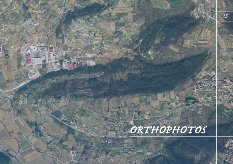
An orthophoto is an aerial photograph that has been geometrically corrected by the rectification process such that the scale of the photograph is uniform, meaning that the photo can be considered equivalent to a map. Unlike an aerial photograph, an orthophoto can be used to measure true distances, because it is an 'accurate' representation of the earth's surface, having been adjusted for topographic relief, lens distortion, and camera tilt.
