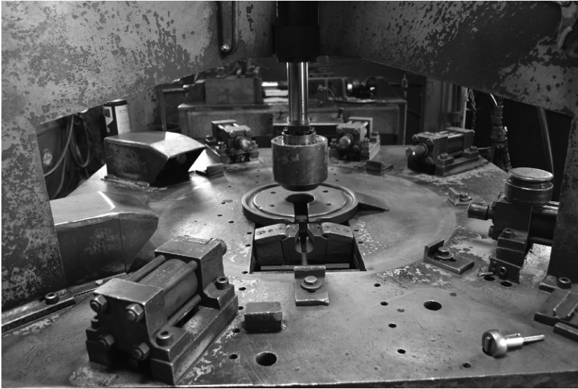
Figure 5.3 Hydraulic machine that Paul designed and built to make metal tractor tires.
