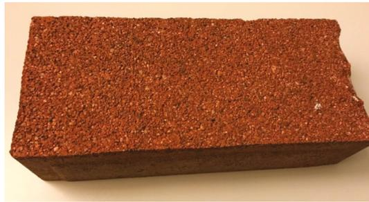
**Figure 2.** Photocatalytic concrete pavement block.
