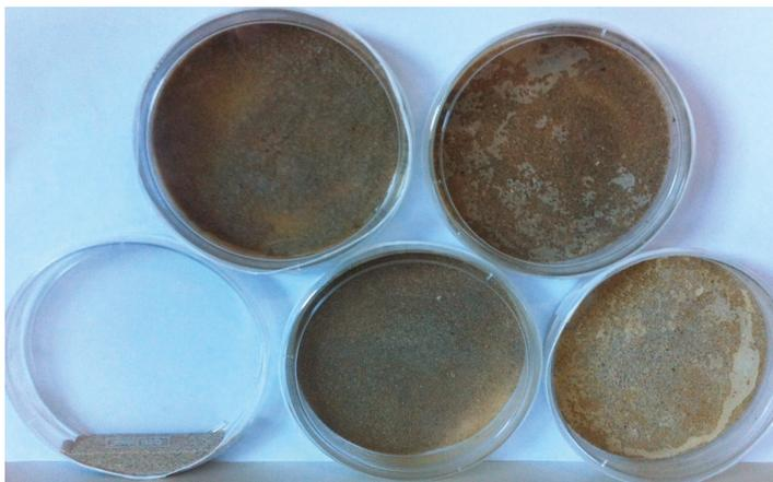
**Figure 6.** Samples of biocemented sand through  $\text{CaCO}_3$  precipitation by strains P2, P11, M5, and P9 (starting from the **upper left** to the **lower right**) after 20 days of incubation, at 28 °C. Untreated control at the **left bottom**. The plates were positioned vertically to highlight the biocementation of the sand, not present in the control.
