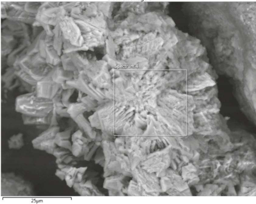
**Figure 10.** EDS spectrum and SEM image of the sand after 20 days of treatment at 28 °C with the strain P9 (*Clavibacter agropyri*).
