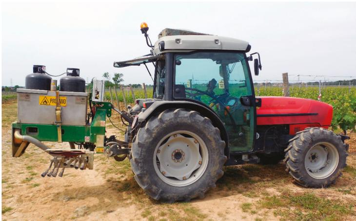
**Figure 2.** The flaming machine PFV-600 (Officine Mingozzi, Ferrara, Italy) coupled with a SAME Frutteto 100 (SAME, Treviglio, Italy) tractor.
