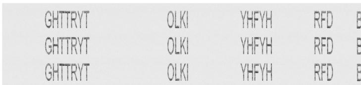
**Figure 20.** Example of reconstructed image from sensitive emission for a two-diode laser printer, 660 dpi mode with the “Eco” option turned on. Measured frequency of sensitive emission:  $f_0 = 444$  MHz,  $BW = 5$  MHz. Image is inverted.
