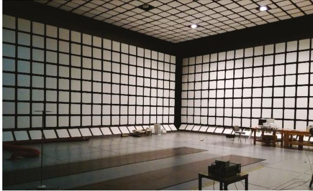
Figure 3. An anechoic chamber.
