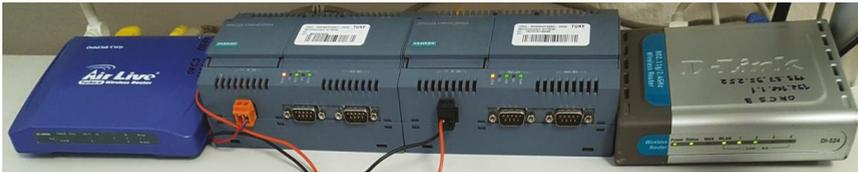
Figure 18. MindConnect devices as gateway to MindSphere cloud.
