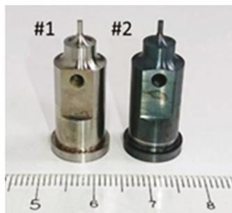
**Figure 12.** Forging punches: #1 uncoated, #2 AlCrSiN-coated.
