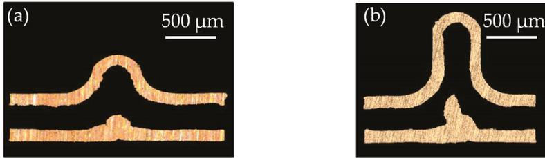
**Figure 11.** Axial cross-section of T-shape samples (C1220) under different MTHF conditions: (a) sample hydroformed at  $p_h = 50$  MPa,  $\Delta L = 450$   $\mu\text{m}$ ; (b) sample hydroformed at  $p_h = 120$  MPa,  $\Delta L = 700$   $\mu\text{m}$ .
