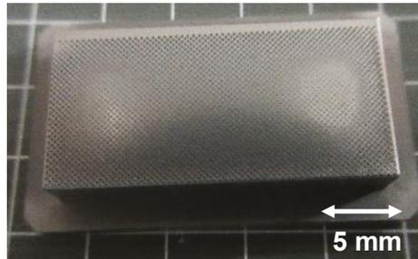
Figure 6. Selectively plasma-nitrided AISI316 die substrate at 673 K for 14.4 ks.
