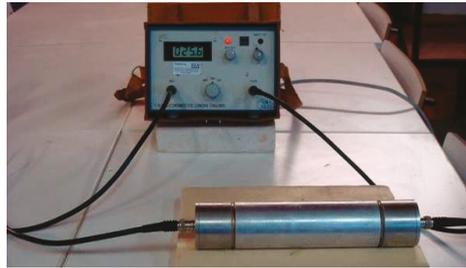
Figure 8. Calibration of the PUNDIT apparatus.
