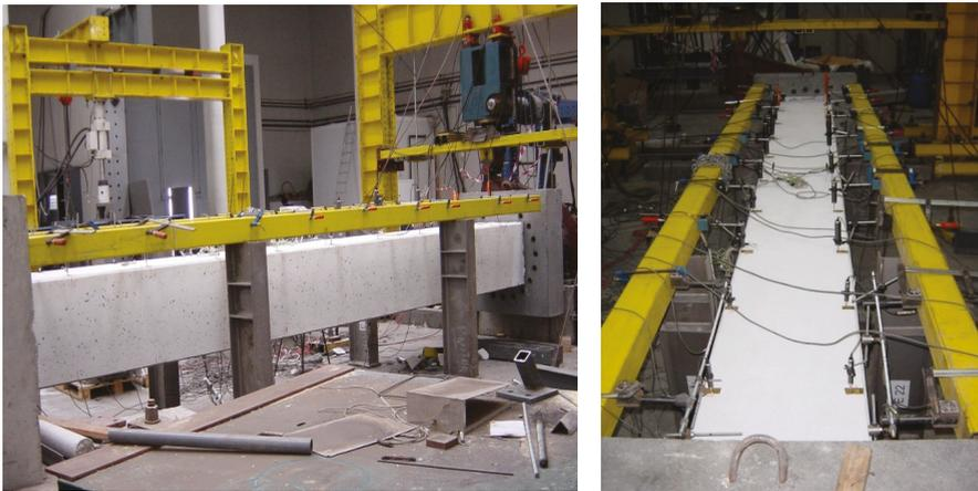
Figure 7. Beam specimen in test position.
