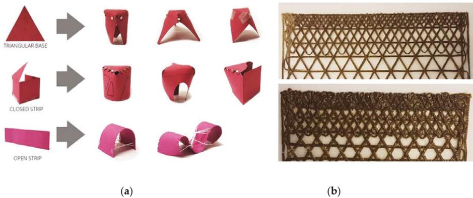
**Figure 4.** Design Process: (a) global design paper models; (b) material test samples with vacuum-infused resin. Top to bottom: 1200 Tex Fibre and 2400 Tex non-twisted roving.
