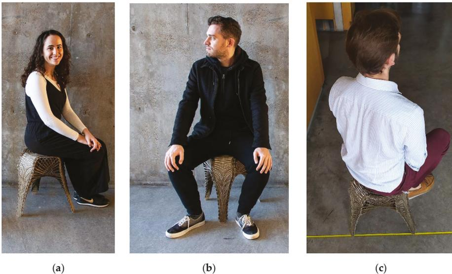
**Figure 13.** Preview of the seating test: (a) 55 kg user; (b) 70 kg user; (c) 85 kg user.
