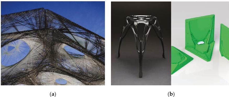
**Figure 1.** Fabrication frames and molds: (a) coreless filament winding (CFW); the Institute for Computational Design/the Institute of Building Structures and Structural Design (ICD/ITKE) Research Pavilion 2013–14 and its module edges shaped by a complex reconfigurable steel filament winding frame [9]; (b) tailored fiber placement (TFP); the L1 Lightweight Stool alongside its elaborate rigid mold [8].
