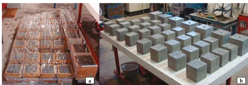
Figure 6. Concrete test specimens: (a) protection, (b) demolding.
